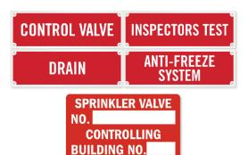
The installing contractor shall also identify a hydraulically designed sprinkler system with a machine engraved weatherproof metal, or rigid plastic sign secured to the riser it serves with corrosion resistant wire, chain, or other approved means. Such signs shall be placed at the alarm valve, dry valve, preaction valve, or deluge valve supplying the corresponding hydraulically designed area.
