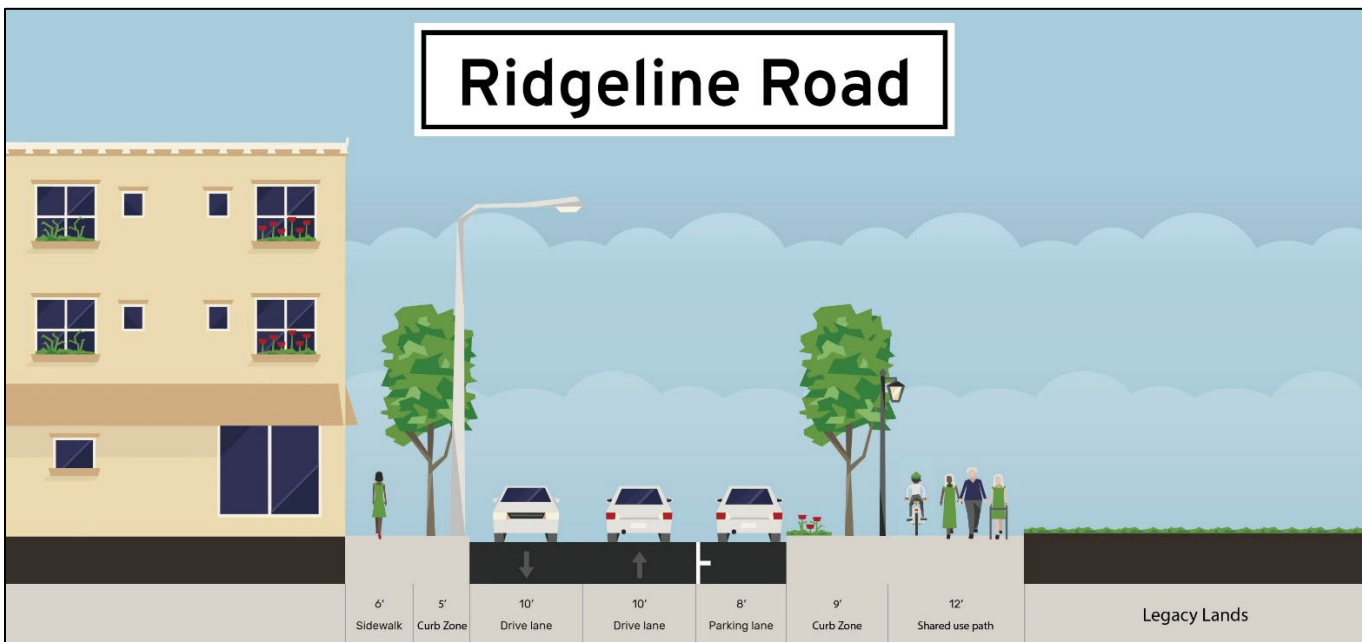
Figure 15. Ridgeline Road – Conceptual Cross Section
