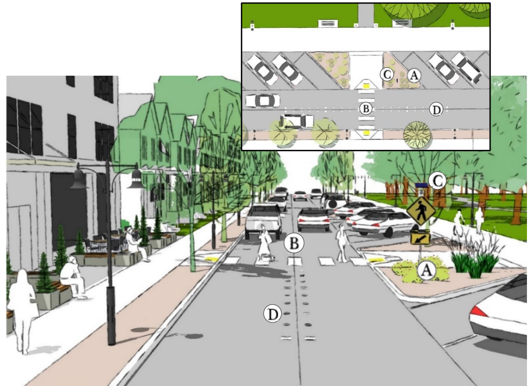
Figure 14 Enhanced Crossing Elements
